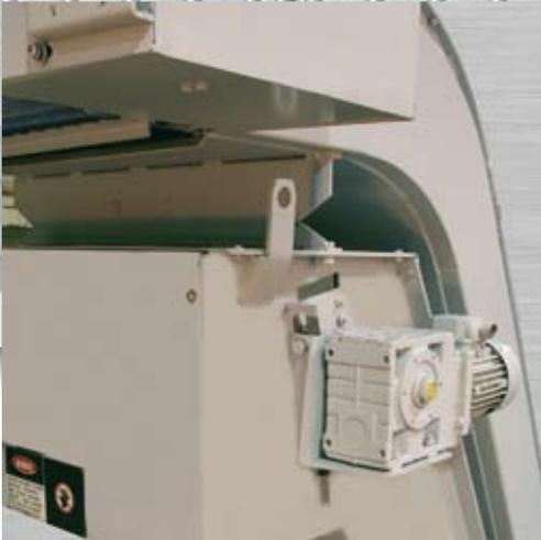
The upper conveyor separates heavy chip loads from the coolant stream. This conveyor efficiently removes chunks, stringy, bushy and large chips and is ideal for multiple material applications. Any small chip or particle passing through the upper conveyor is trapped in the lower filtering conveyor. High speed aluminum machining is one of the many applications ideal for the Turbo MF2/MF3.
